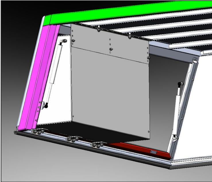
Fit the 3 off bottom brackets to the canopy nut slot frame using the supplied M8x20 bolts, nylock nuts and washer fasteners. Slide the M8x20 bolts into the nut slot frame of the canopy (2 per mounting bracket).
