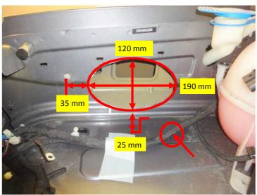
Mark section as shown in the image and cut it using hole saw. Remove excess wiring harness holder (arrow).
