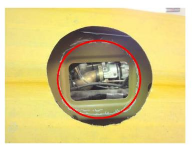
Through the fender breakthrough, mark the magnification on the engine compartment partition wall along the edge using a pencil, and cut it off.
