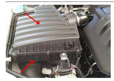
Reconnect water drain hose to the bottom air filter housing provided in the delivery.
