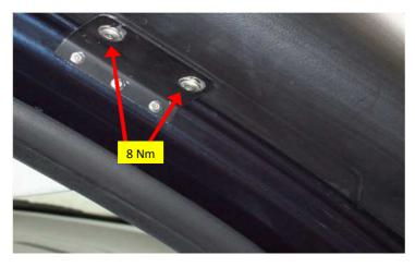
Screw the bracket with the pipe, do not completely tighten the screws as yet.
