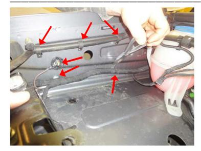
Loosen the wiring harness, earth strap as well as water hose in the engine compartment on the right and place aside.
