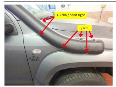
Tightening torque in Nm.
