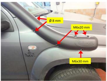
Align snorkel pipe to mud guard using 3x M6x20 and 1x M6x30 with washers and nuts and fasten temporarily. Mark both the missing drill holes while the snorkel pipe is fitted tight, and remove the snorkel pipe again.
