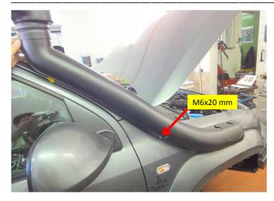
Align snorkel pipe to mud guard using 3x M6x20 and 1x M6x30 with washers and nuts. Screw in both the missing screws M6x20 mm in the rivet nuts, align snorkel pipe to a-pillar and tighten both the screws at the top.
