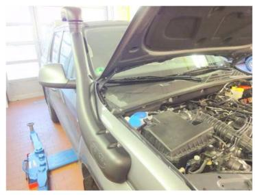
Fix both the air filter housings, mount all the hose connections back to their original points and complete the wheel house again on the right.
