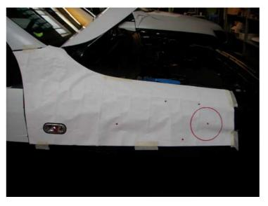
Place the drill template on the fender and align to the outline of the fender and fix. Using template, transfer all 4 screw holes and air pipe breakthrough onto mud guard. Make air pipe section (ø 120 mm) and the 4 holes (ø 7 mm). Deburr all edges, remove drilling chips and swarfs and treat the cutting edges against rust.
