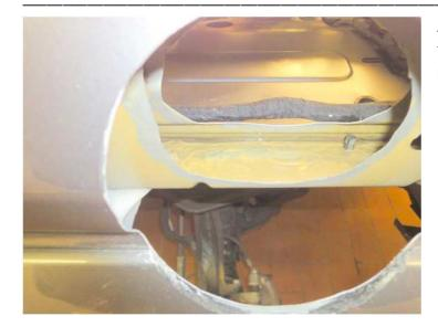
After sealing all the cutting edges, treat all the hollow spaces with suitable hollow space protection wax.
