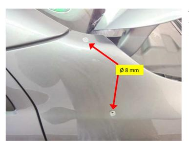
Take off snorkel pipe, drill the marked holes to 8 mm and insert 2 rivet nuts M6 using rivet nut pliers.
