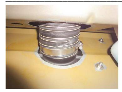
Position the air filter housing through the countersunk opening to the snorkel pipe, place the hose fitting without any friction and fix to snorkel pipe using hose clamp.
