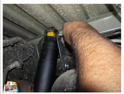
Unpack new Old Man Emu shock absorber and fit to upper mount using original equipment bolts.
