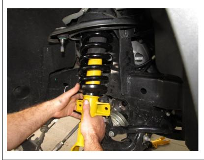
Refit strut assembly. Lubricate rubber top hat and CV joint boot to allow clevis to slide past CV boot.
