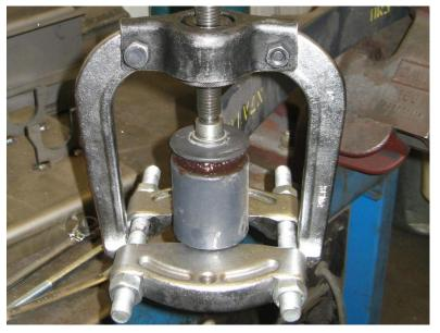
Fit the bearing separator and puller to the new spring.
