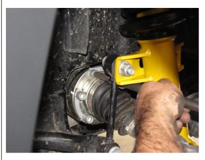
Re align driveshaft using the marks made earlier. Replace driveshaft bolts and washer plates.
