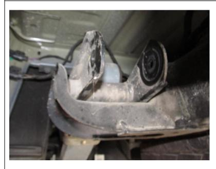
Swing shackle towards rear of the vehicle to create extra clearance to aid spring removal.
