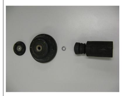
Once strut is disassembled, retain the original dirt shield/bump stop, washer, top hat and top rubber spacer for re fitment to Old Man Emu Strut.
