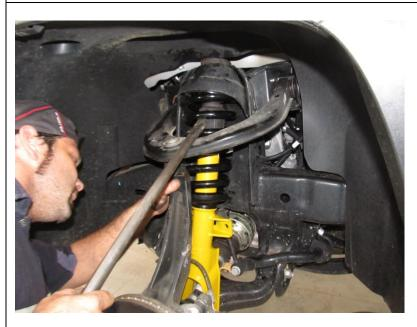
Using the lever bar in the top arm, align the upper arm ball joint. Replace nut and torque to manufacturer's specification.
