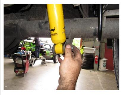
Lower vehicle slightly to align shock absorber bottom mount. Secure with original bolt and nut.
