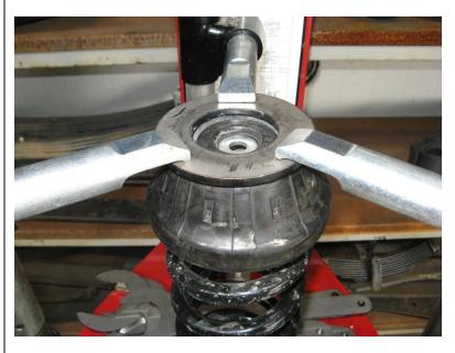
Before disassembly place the coil spring ring from the FK33 Amarok workshop fitting kit on top of the strut assembly
