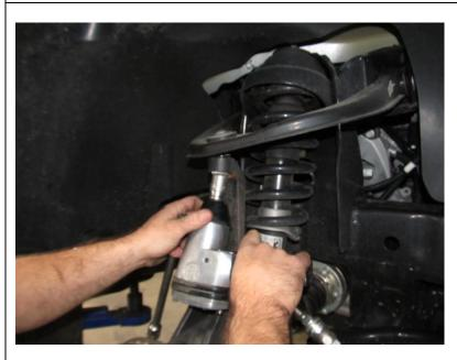
Remove upper arm ball joint nut. With assistance from another person release taper on ball joint with ball joint puller whilst holding hub assembly.
